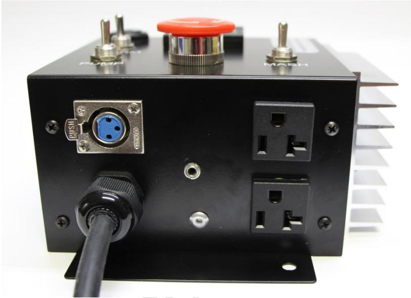
**Main incoming power at bottom left corner.** If you purchased a 120V controller this will be an 8 foot power cord that will have a standard 3 prong plug or depending on options, a GFCI plug. If you purchased the 220/240V 30 Amp controller this will be a 12 foot 10 Gauge power cord with a 4 prong dryer style plug on the end.
